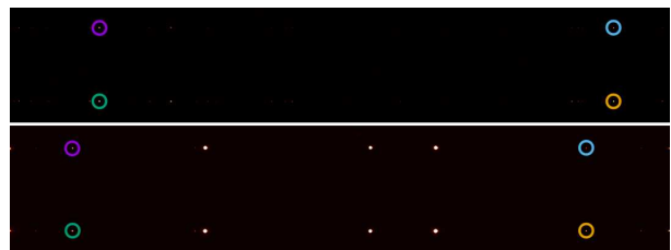
Fig. 11. Anchor images captured by the two cameras. The four circled emission spots correspond to the specific monitoring regions used during the focus alignment procedure. The pixel positions of these spots are subsequently referenced as master spatial and spectral coordinate origins to determine the precise locations of the entire scientific spectra on the detectors. Alt text: Two detector images, each showing two parallel columns of emission-line spots arranged horizontally near the top and bottom of the frame, with four specific spots highlighted by circles.
