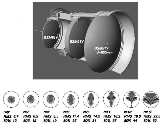
Figure 3. The optical and mechanical design of the prime focus corrector optics. The spot diagram of the corrector at zenith distance of 0 degree at wavelength 0.9, 1.37, and 1.8 \mu\text{m} is shown at bottom. The circles represent a diameter of 100 \mu\text{m} , and RMS spot sizes and 80% encircled energy diameters are listed in \mu\text{m} . Note that 83 \mu\text{m} corresponds to 1'' .
