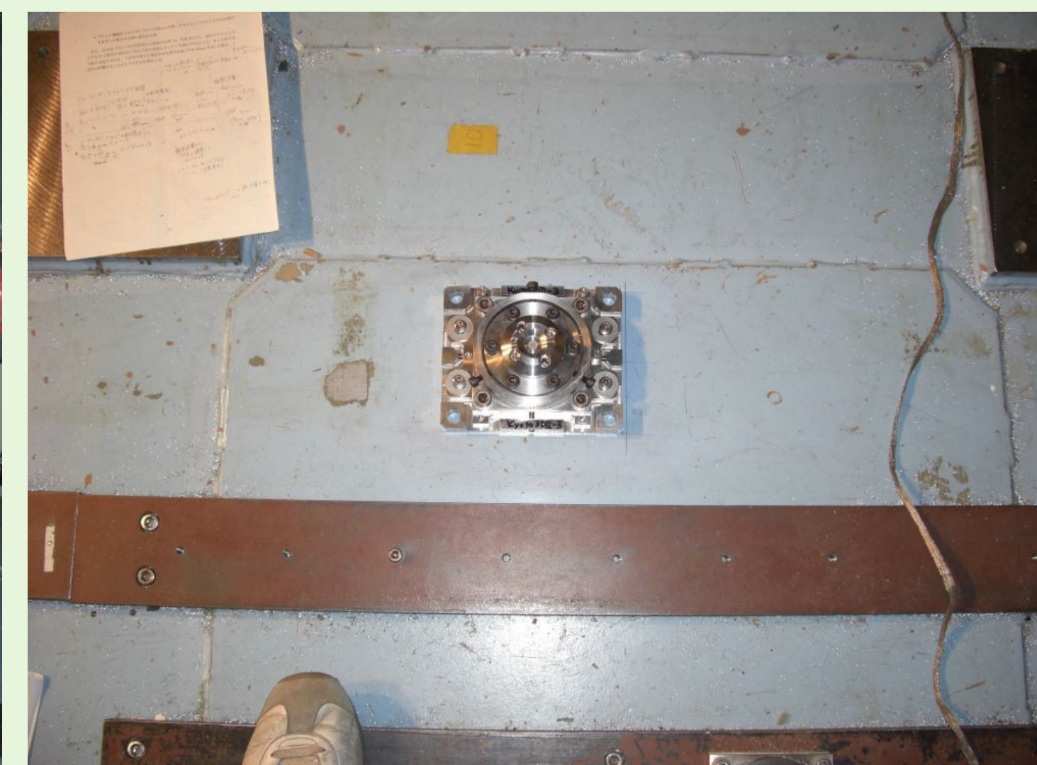
Measured the relative position to the output light axis of the AO188 and positioned our fixed point mount.
